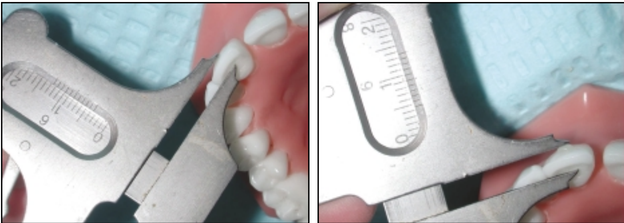
Fig. 3 Before-and-after Boley gauge readings used to measure exact height of bonded composite mound.
